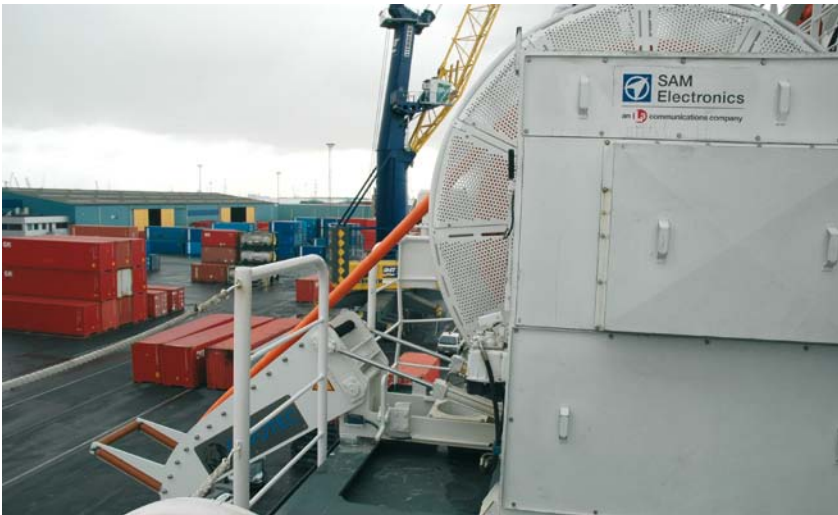
Cable reel with swung out cable guide
