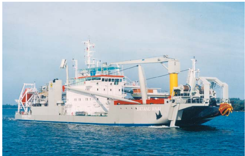
Cutter suction dredger "Batang Anai"
